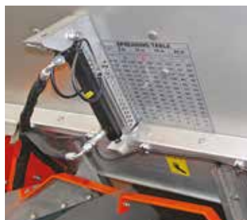
Double acting hydraulic control of fertilizer flow
